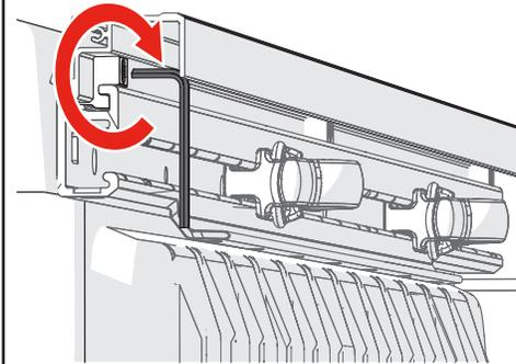
**13** Attach the rail end caps (M) to the adapter rail (H) with the flat rail end cap screws (N).
