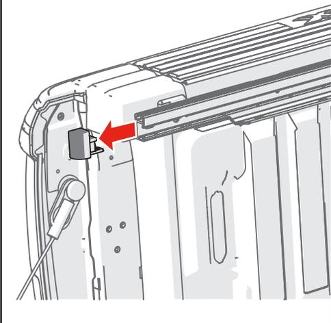
**6** Place the adapter rail (H) into the top of the factory accessory rail and slide it toward the cab.
