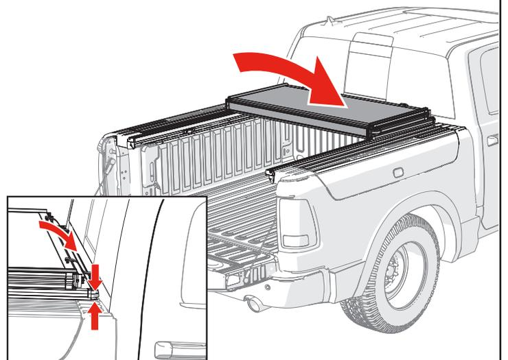
**NOTE:** When placing the cover (A) onto the bulkhead the corner seal will slide down in front of the cover rail.
