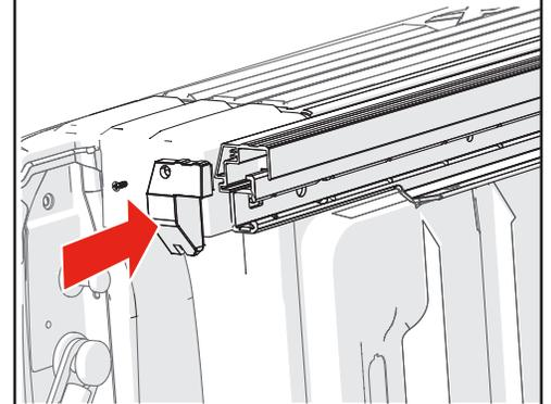
**14** Adhere the ribbed D-seal (L) in the end cap corner to span the adapter rail (H) end cap and rear trim panel. Add one to each side. Trimming the seal may be required.
