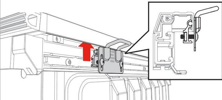
**21** Close the cover (A) and align the striker bracket (B) with the bed cover latch. Push down on the cover while tightening the Torx screws (E).
