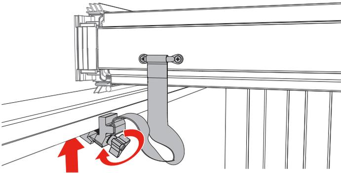
**19** Close the tailgate and unfold the cover. Check that the cover is parallel and square with the truck bed and bed rails. If not parallel or square, open the cover and loosen the cab clamps to reposition the cover. Adjust and re-tighten both clamps.
