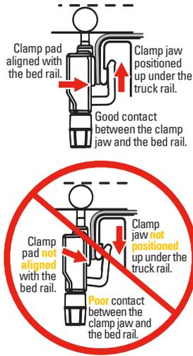
**17** Do Not use a wrench or overtighten. Hand tighten until the clamp jaw contacts the adapter rail (H), then tighten an additional two turns.
