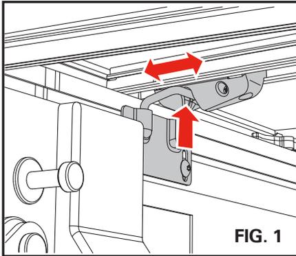
Lower the rear of the bed cover and adjust the position of each latch so that they engage with the striker brackets, (**Fig. 1**). With the latches adjusted, from underneath the cover, use the provided T-20 Torx wrench to tighten the two screws, (**Fig. 2**) in both the driver and passenger side latches.
