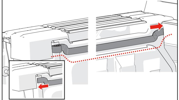
**3** Place the flat D-seal (K) to continue the flat seal (I) across the back end cap.
