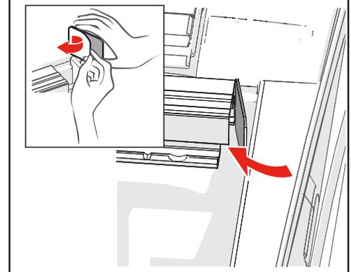
**8** Slide the adapter rails (H) and the rail end seals (J) firmly against the bulkhead.
