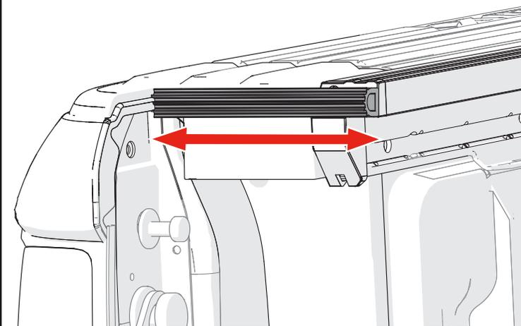
**15** Place the cover (A) onto the truck bed rails and bulkhead. **NOTE:** Take care not to damage or deform the cover seals while installing the cover.
