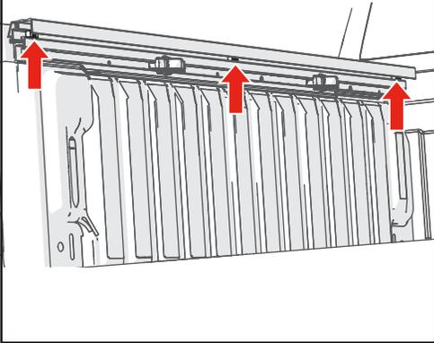
**12** With the adapter rail (H) firmly pressed up to the bulkhead, tighten each lock block (F) with the 3/16" hex wrench provided.
