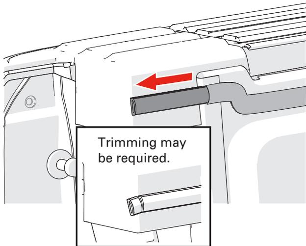
**4** With the seals (I & K) in place on both sides, reinstall the factory accessory rails.
