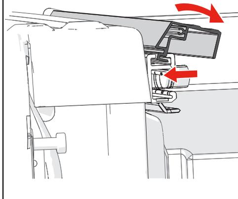
**7** Before the adapter rail (H) is slid completely to the bulkhead, remove the backing and attach a rail end seal (J). Do this for both sides.
