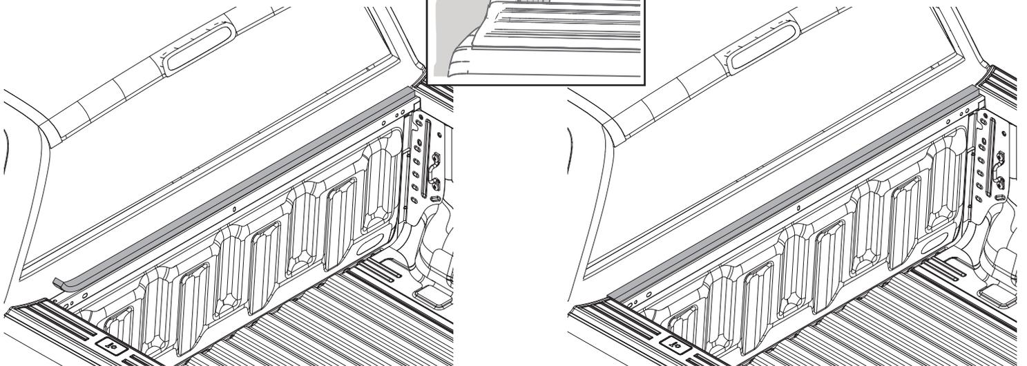
**4** Place the assembled bed cover (A) over the cab end of the truck bed. **NOTE:** Take care not to damage or deform the seals when installing the bed cover onto the truck bed. Visually check to ensure the front bed cover frame is even on both sides and square with the bed. Make sure the cover is centered on the bed of the vehicle before tightening clamps.
