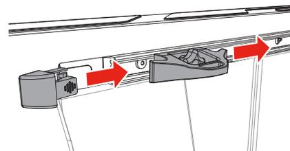
Reinstall any tie-down cleats and the end cap on both sides of the truck.
