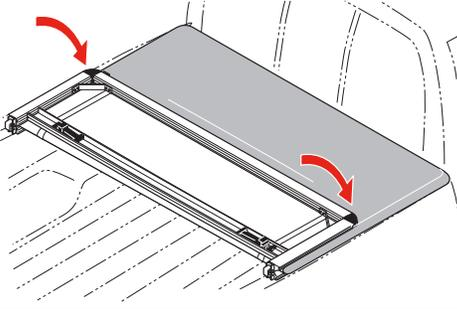
**IMPORTANT:** Before folding the second section of the tonneau, the rear clamps must be stowed into the rail to prevent damage to the fabric. **Failure to stow the handle will puncture the tarp and void the warranty.**
