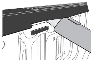
Trim the plastic high enough to expose the truck metal, and wide enough to accommodate the clamp.
