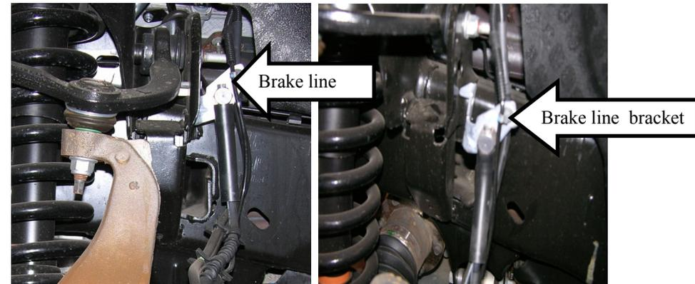
4. Separate the upper ball joint from the spindle. Use a ball joint separator or other suitable tool.
