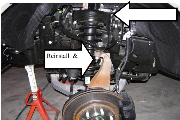
12. Reinstall the brake line bracket to the strut tower.
