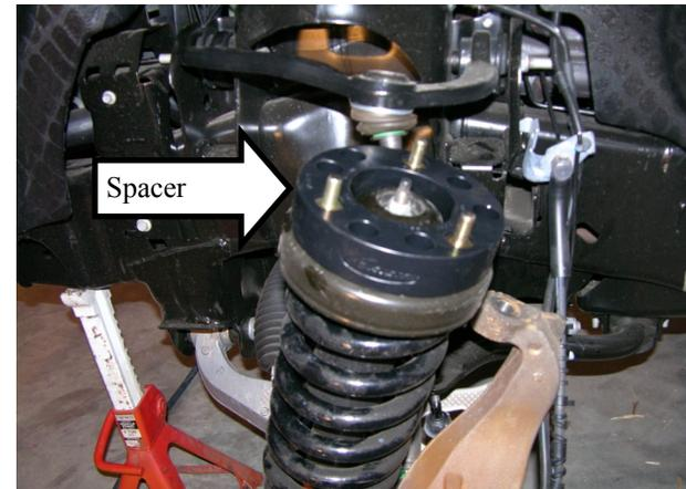
9. Push the upper control arm up and push the strut inward and place the jack under the lower control arm and jack up so the strut studs will go through the strut tower, use the new lock nuts and washers to install the strut.
