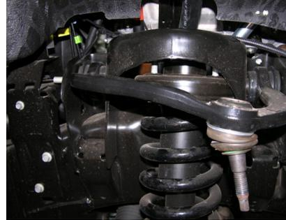
6. Loosen the lower strut bolt and nut and push the upper control arm up and pull the strut toward you.
