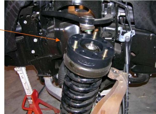
10. Push the upper control arm up and push the strut inward and place the jack under the lower control arm and jack up so the strut studs will go through the strut tower, use the new lock nuts and washers to install the strut.
