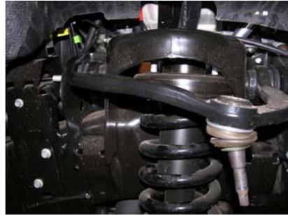
7. Loosen the lower strut bolt and nut and push the upper control arm up and pull the strut toward you.
