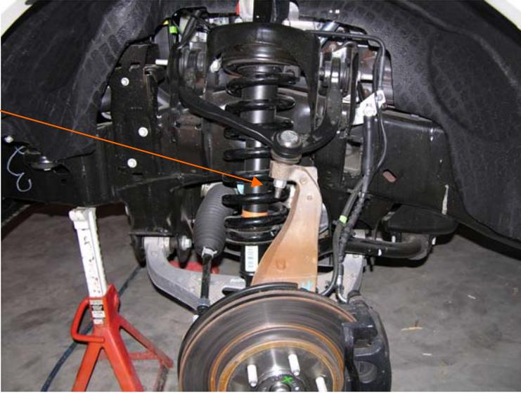
13. Reinstall the brake line bracket to the strut tower.
