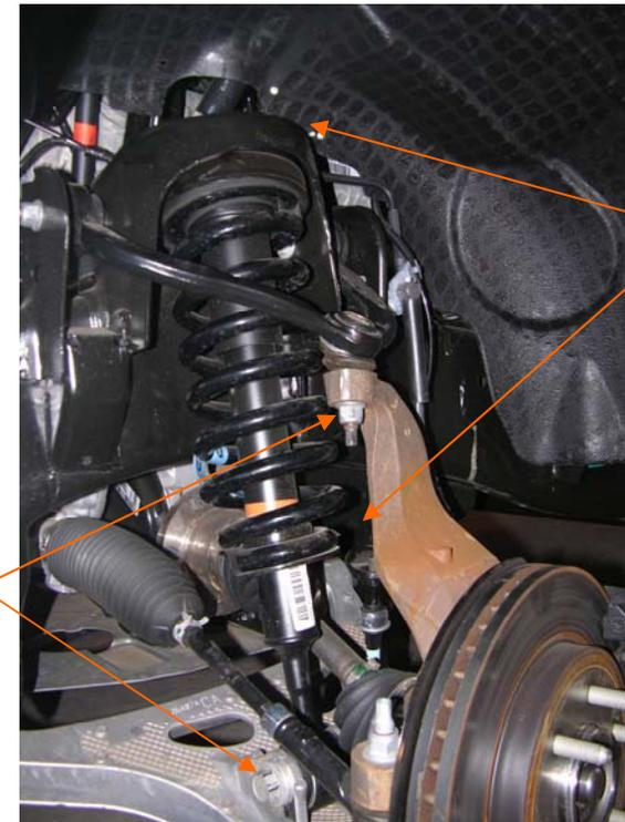
12. With the ball joint nut installed on the ball joint tighten the upper strut nuts.
