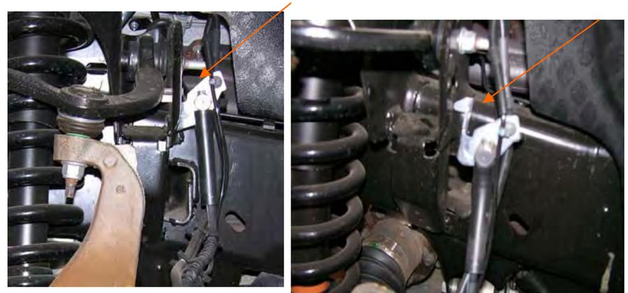
5. Separate the upper ball joint from the spindle. Use a ball joint separator or other suitable tool.
