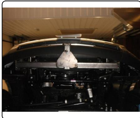
6. Insert spacer plate (6) between the frame and hitch side plate. Insert two 5/8" x 4" hex bolts (1) with a lock washer (2) and washer (3) on each. Insert in through the side plate / spacer and out the frame, as shown on page 2. Attach using two 5/8" hex flange nuts (4), two spacers (6) and repeat on the other side.
