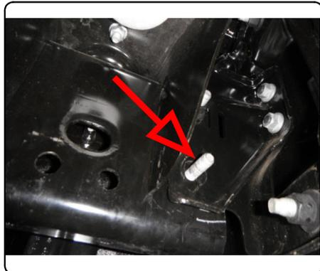
3. Loosen the top nut on each side until only a couple threads are engaged. The top nut will prevent the bolts from being pushed completely through. Push both sets of bolts towards the center of the vehicle.
