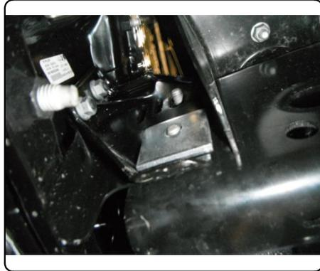
5. Raise the hitch into position by first raising the passenger side of the hitch and inserting the bolts back into position through the forward most hole in the hitch side plate. Rotate the driver side of the hitch up into position and push the bolts back towards the outside of the vehicle.
