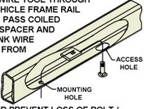
INSERT COILED END OF FISHWIRE TOOL THROUGH HITCH MOUNTING HOLE IN VEHICLE FRAME RAIL AND OUT THE ACCESS HOLE. PASS COILED END OF FISHWIRE THROUGH SPACER AND THREAD BOLT INTO COIL. KINK WIRE TO KEEP SPACER SEPARATE FROM BOLT AS SHOWN. PULL FISHWIRE, SPACER, AND BOLT THROUGH FRAME AND OUT MOUNTING HOLE. USE FISHWIRE TO GUIDE HITCH DURING MOUNTING AND PREVENT LOSS OF BOLT / SPACER INSIDE FRAME RAIL.
