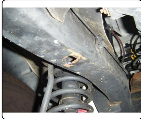
4. Fishwire (2) carriage bolts and (2) SP-6 spacers into position in the side of each frame rail. Reverse fishwire (1) carriage bolt and (1) SP-6 spacer into position in the bottom of each frame rail. NOTE: Leave fishwires attached to all hardware to prevent losing in frame.
