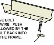
ATTACH FISHWIRE TO CARRIAGE BOLT AND SLIDE SPACER ONTO FISHWIRE. PUSH THE BOLT THRU THE HOLE FOLLOWED BY THE SPACER (AS SHOWN). PULL BOLT BACK INTO POSITION, PROTRUDING FROM THE FRAME.
