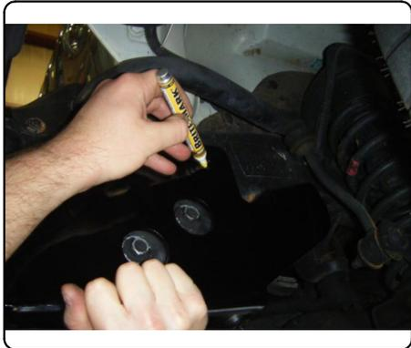
2. Lower hitch and drill (2) holes using a 9/16" drill bit.
