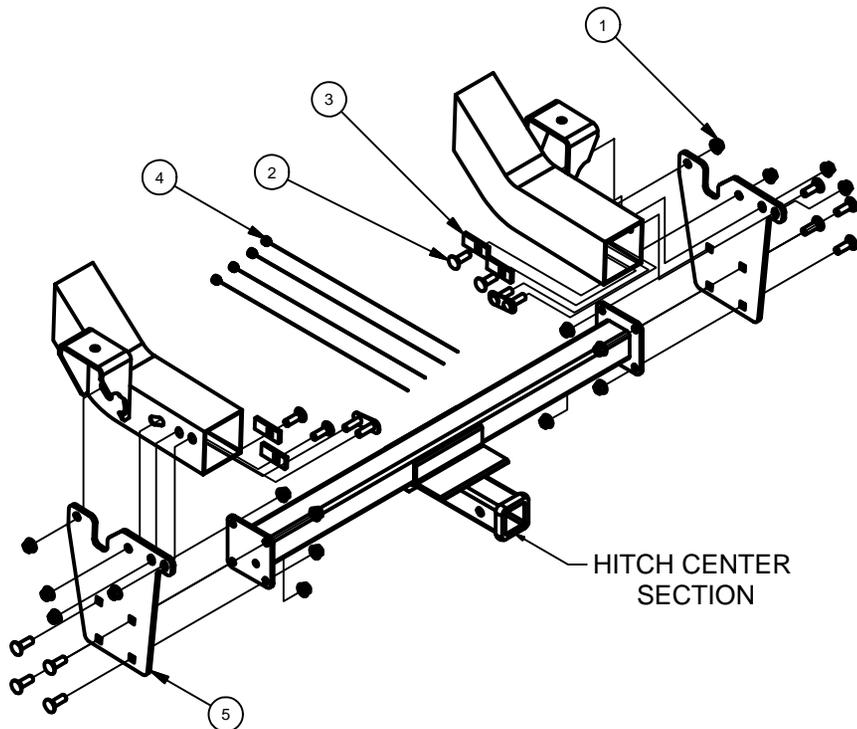
1. Use 18mm socket and ratchet to remove driver and passenger side tie down brackets if present. Existing bolt plates will fall out of front of frame rails.
