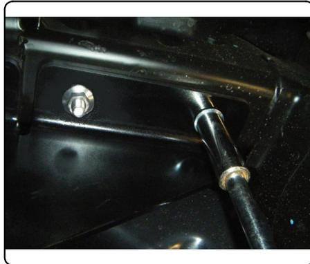
9. Hitch shown installed properly.
