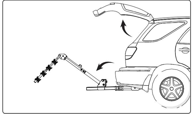
At the top, pull the lynch pin that secures the arms in the outward position. Fold the bike rack arms down to the transport position, and replace the lynch pin.
