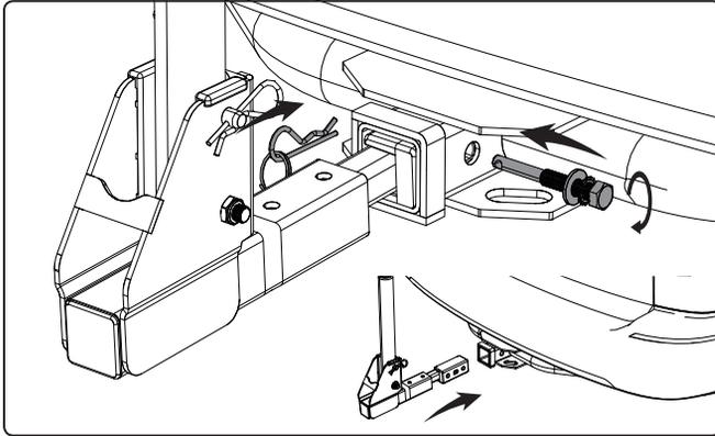
**Note:** To adapt the 1 1/4" shank to fit a 2" receiver tube opening, assemble the U-type adapter (#5) onto the 1 1/4" shank (#4). Align the holes and secure with 1/2" hex head bolt, flat washer, star washer and clip (#11).
