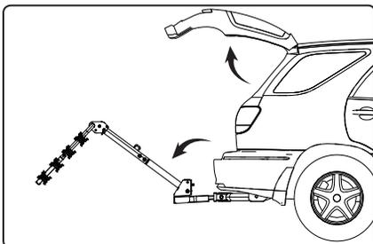
At the base, remove the clip from the upper bolt holding the bike rack in the vertical position. Remove the bolt and tilt the rack away from the vehicle. The rear cargo area is now accessible.
