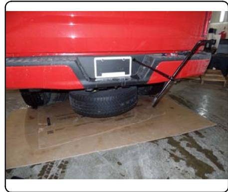
2. For the rearward most holes, tape a U-shaped spacer into the recess in the frame. Thread the forward most fishwires through another rectangular spacer on each side and then thread all of the fishwires through their appropriate mounting holes.
