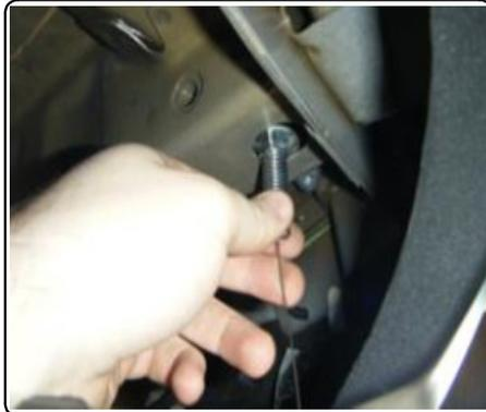
5. Raise hitch into position and secure with supplied M12 hex bolts and 1/2" conical toothed washers into existing vehicle weldnuts. Secure 1/2" carriage bolt with supplied hex flange nut.
