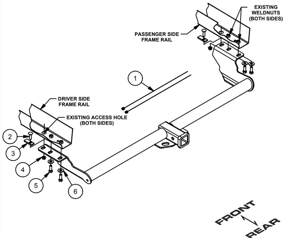
1. If present, remove (6) fasteners ((4) plastic push pins, (1) phillips head screw and (1) hex bolt with 10mm socket) and the plastic underbody panel covering the driver side frame rail. Return fasteners and plastic shield to owner. Remove (2) fasteners on the exhaust deflector and temporarily remove deflector.
