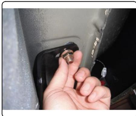
5. Torque all 12mm hardware to 86 lb-ft and all 7/16" hardware to 70 lb-ft. Reinstall exhaust deflector.
