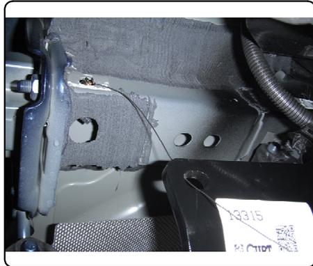
8. Insert M12 bolts with conical toothed washers. Be sure the tooth side of washers are against the hitch and the 1/2" flat washers clamped in position between the hitch and frame rail.
