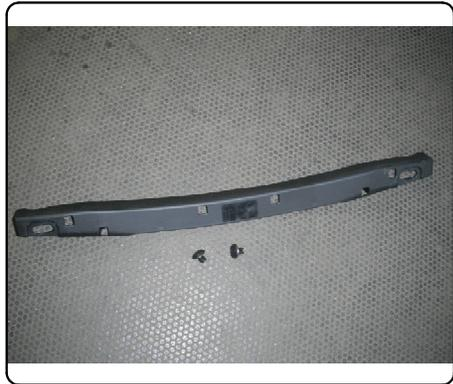
2. Remove tape on the side of vehicle frame rails to expose mounting locations. Trim any excess seam seal (if it will interfere with hitch).
