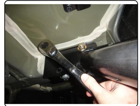
6. Torque all 1/2" hardware to 110 ft-lbs. Torque all 10mm hardware to 48 ft-lbs. Raise exhaust and spare tire back into position. Reinstall passenger side and driver side under body panels removed in Step (3).
