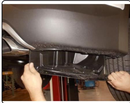
4. Raise hitch into position and secure to the existing weldnuts with M10-1.25 x 25mm bolts and 3/8" conical toothed washers. **Note:** The bumper locator pin may interfere with the hitch hardware. You may need to bend or trim it to allow hardware clearance.
