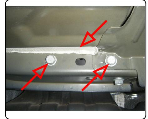
2. Raise hitch into position and reinstall (4) M14 bolts. Torque all M14 hardware to 126 ft-lbs.
