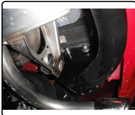
5. Align the bottom tabs of the hitch with the weldnuts in the frame rails and secure with M10-1.25 x 25mm bolts and 3/8" conical toothed washers.
