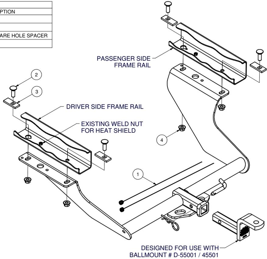
REMOVE PLUG AND MODIFY USING DIE GRINDER (OR ROUND FILE) TO ALLOW INSERTION OF 1/2-13 BOLTS AND CM-SP10 SPACERS INTO FRAME RAIL
