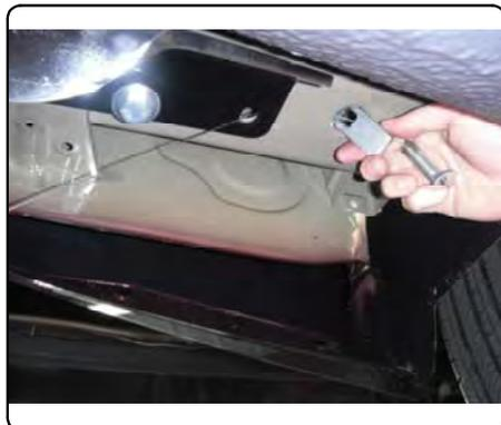
5. Torque all 12mm hardware to 11 ft-lbs. Torque all 7/16" hardware to 10 ft-lbs.
