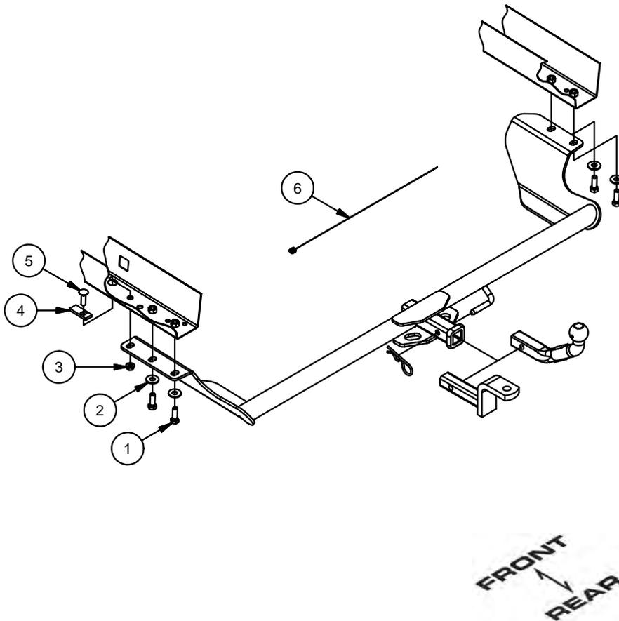
1. If present, remove (5) fasteners and the plastic fascia covering the driver side frame rail. Return fasteners and plastic fascia to owner. **Note:** You may trim fascia and re-attach after hitch installation.
