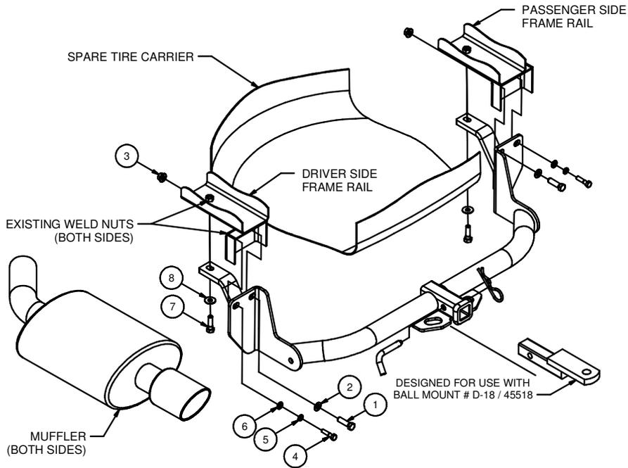
1. Lower the exhaust by removing the (3) rear most rubber isolators on each side of the exhaust. Gently spread the exhaust to allow the mufflers to pass by the spare tire carrier. Support the exhaust system to prevent damage. (See Rubber Isolator Removal Diagram.)
