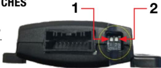
In the illustration above, the switch on the right (#2) controls the level of output available to the trailer brakes when using the manual control. The factory default setting is the 'ON' position with the switch down. This setting limits the manual control output to the level set using the output control. Moving this switch up to the 'OFF' position allows 100% of the output to the brakes when the manual control is actuated regardless of the output control setting.
