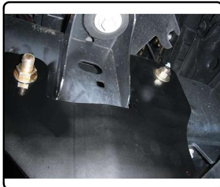
5. Torque all 1/2" fasteners to 110 lb-ft and all 5/8" fasteners to 180 lb-ft.
