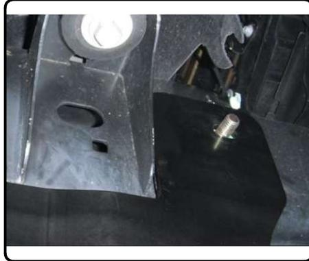
4. Fishwire the 5/8" carriage bolts from the end of the frame into the rearward mounting slots in the frame. Loosely install the remaining 5/8" hex flange nuts.
