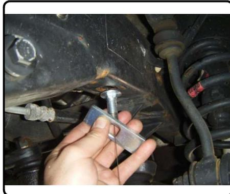
5. Thread fishwires through hitch mounting holes and raise hitch into position. Secure to frame using 1/2" flange nuts.
