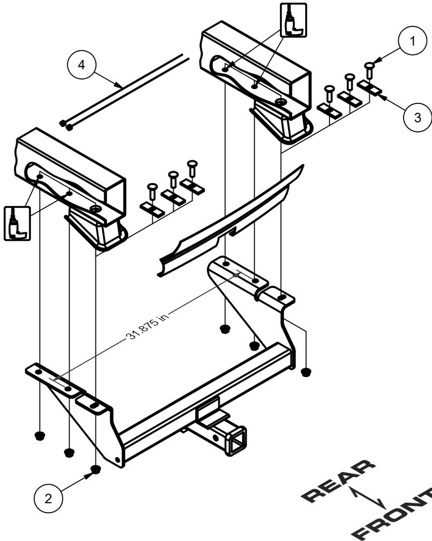
1. Determine if trimming is required on model by raising hitch into position. If needed, mark and trim lower fascia or remove lower fascia and return to owner. (See fascia trim detail) **Note:** Check for proper fit prior to trimming.
