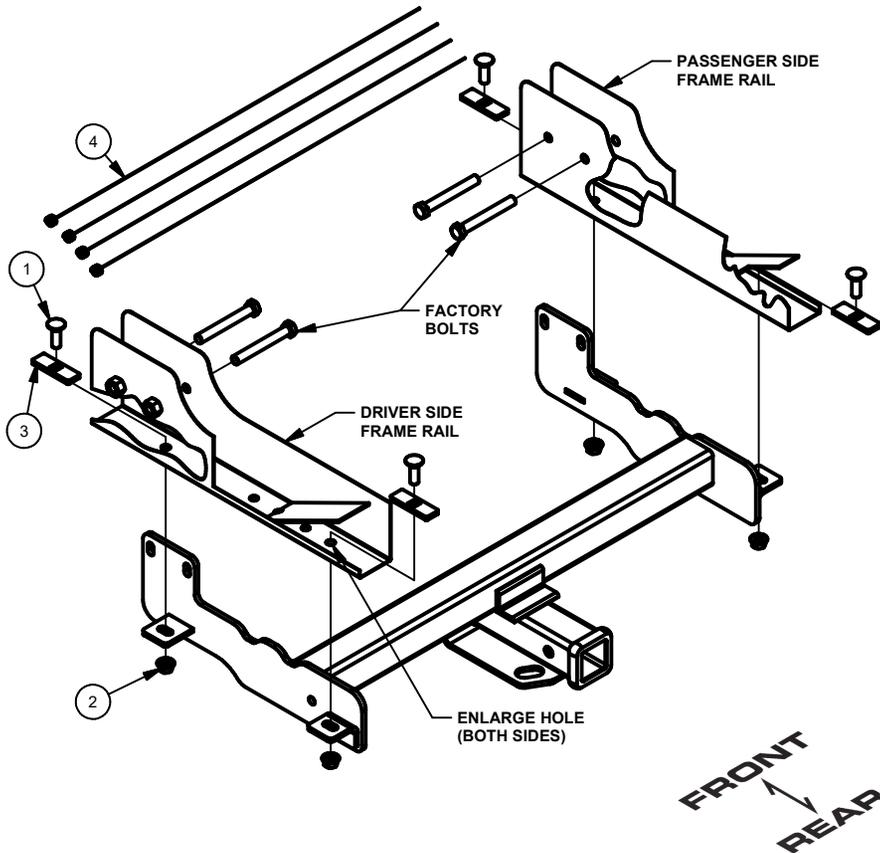
NOTE: Lower spare tire for ease of installation.
