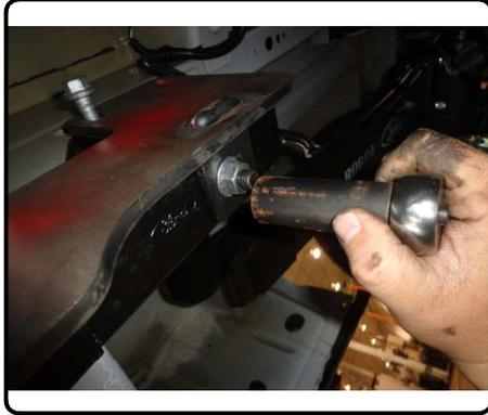
4. Torque M12 fasteners to 90 ft-lbs and all 1/2" fasteners to 110 ft-lbs. Re-install spare tire if lowered.
