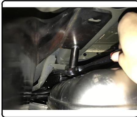
5. Torque all 7/16" hardware to 59 ft-lbs and all 1/2" hardware to 110 ft-lbs. Reinstall items removed in Steps 1.
