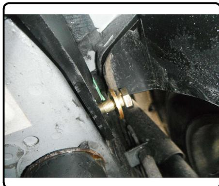
9. Pull 1/2" hardware into position & remove fishwire(s). Fasten with 1/2" hex flange nut(s). Re-secure harness which was unfastened in step 3. Wrap cable tie(s) around hitch mounting plate(s) and harness. Pull tight & trim excess cable tie.
