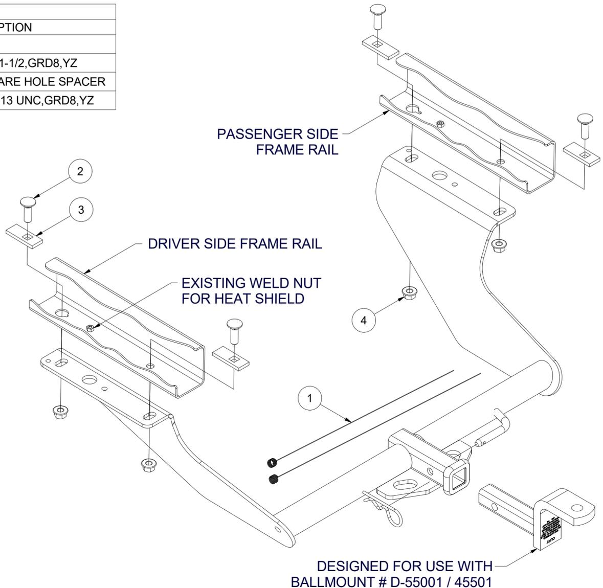
REMOVE PLUG AND MODIFY USING DIE GRINDER (OR ROUND FILE) TO ALLOW INSERTION OF 1/2-13 BOLTS AND CM-SP10 SPACERS INTO FRAME RAIL
