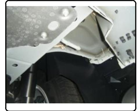
2. Remove heat shield from driver and passenger side of vehicle. The passenger side shield will need (3) screws and (1) plastic plug removed. The driver side shield will need (3) screws, (1) plastic plug, and (1) plastic clip attaching the heat shield to the wiring harness removed.
