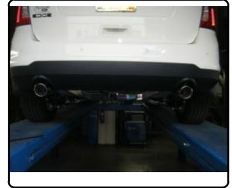
6. Using the hitch as a template, drill the rear holes through the frame rails. Fishwire 1/2-13 x 1 3/4" carriage bolts and CM-SP19 spacers into position and secure with flange nuts.
