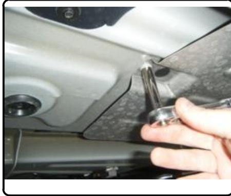
4. Fishwire 1/2-13 x 1 1/2" carriage bolts and CM-SP19 spacers into position through end of frame rails and out mounting holes.
