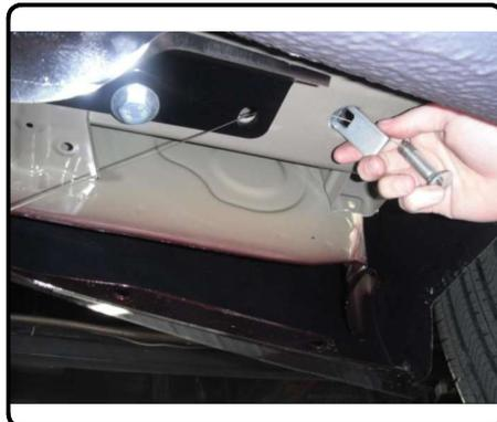
5. Torque all 12mm hardware to 86 ft-lbs. Torque all 7/16" hardware to 59 ft-lbs.
