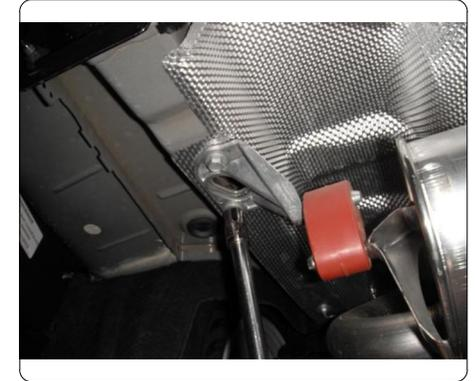
2. Raise hitch into position and temporarily secure to existing weldnuts in the frame rails using M8-1.25 hex bolts and 3/8" conical toothed washers. Using the hitch as a template mark drill location on both sides. Lower hitch and drill holes.
