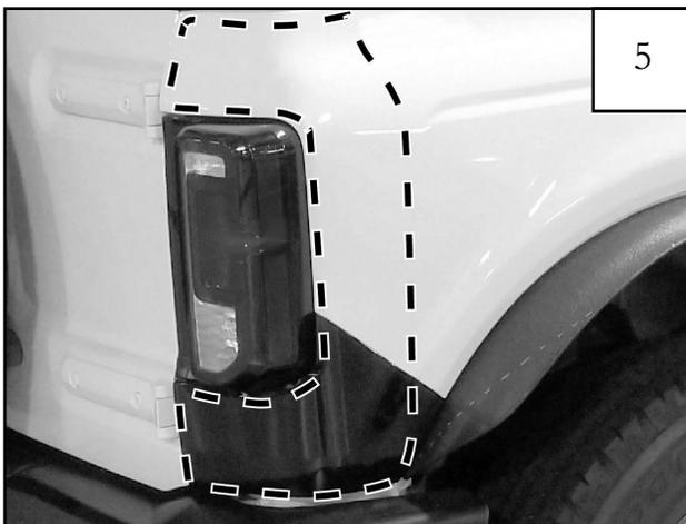
Clean the surface where the tape will contact the vehicle body using the enclosed alcohol pads.
