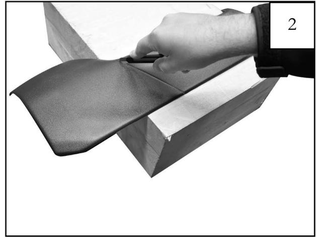
Place Trail Armor Corner on a stable surface and carefully use a utility knife or other cutting utensil to trim along the indented line.
