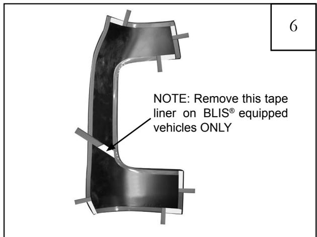
Peel back 2" of red tape liner on all flanges to expose adhesive and create a pull tab.
