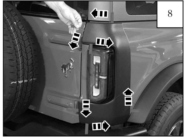
With the Corner Guard in its final position, begin pulling tape tabs to remove remaining tape liners. Proceed in a clockwise pattern, beginning with the upper left hand side as shown above.
