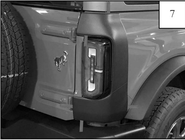
Position the Corner Guard in place and align with the previously cleaned surface. Ensure that the red tape pull tabs are all accessible. Apply pressure to exposed tape.
