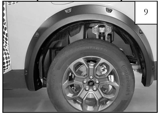
Completed rear fender flare installation.
