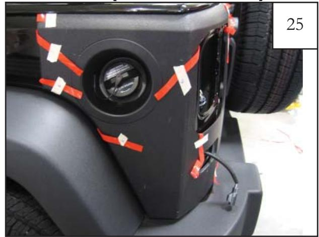
Position the part on the vehicle so it fits around the gas door. Then, using a #2 Phillips screw driver, reattach the tail light.
