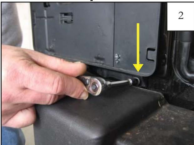
Remove license plate, then using a 7mm socket with a 1/4" ratchet and 1/4" extension, remove two bolts from the bottom of the license plate frame.
