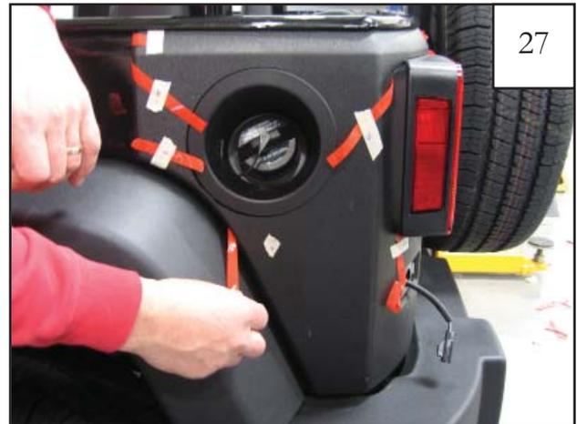
Pull tape liner 2 downward on a slight diagonal matching the curvature of the part. **NOTE:** Refer to step 24 for tape liner tab numbering.
