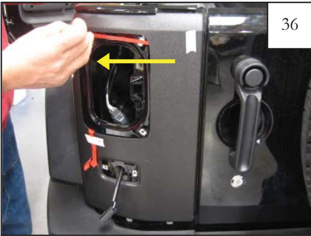
36 Pull tape liner 9 for the 1/4" tape to the left toward the driver side of the vehicle. *NOTE: Refer to step 24 for tape liner tab numbering.*
