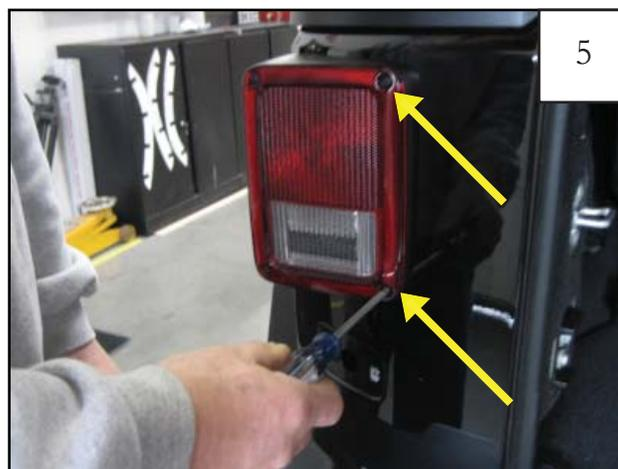
Using a #2 Phillips screwdriver, remove two screws closest to the inside of the vehicle.
