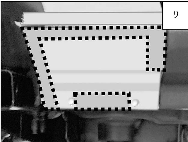
(1) Use alcohol pads to clean areas where the tape on the back of the Trail Armor will contact surface. Let dry.
