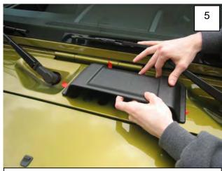
Hold the part at an angle to prevent tape from prematurely sticking, and align the part on the hood using marks made in Step 3 as a guide. NOTE: If necessary, lift windshield wiper out of the way.
