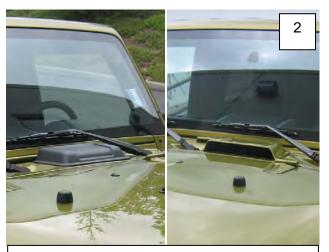
Without peeling liner from tape pads, position the part on the vehicle hood, centering over the air intake grill. You can position the hood scoop with the intake facing front or back as desired.
