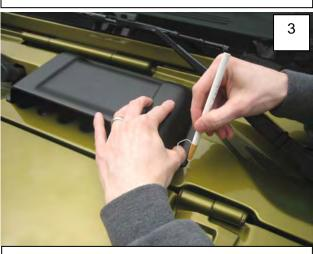
Once positioned, use a grease pencil to lightly trace around edges of part.
