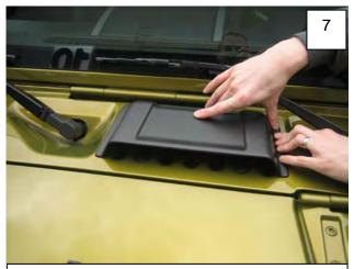
Press part into place. Apply 30 PSI to the taped areas for proper bond. The tape reaches maximum adhesive bond after 24 hours of contact. Do not wash vehicle for 24 hours.
