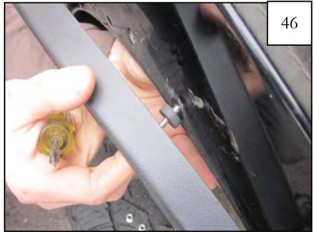
Install inner piece D3 (and P3 for passenger side installation) by lining up the M5-.8 machine screws (SW1-0053) with the factory hole locations and push into place.
