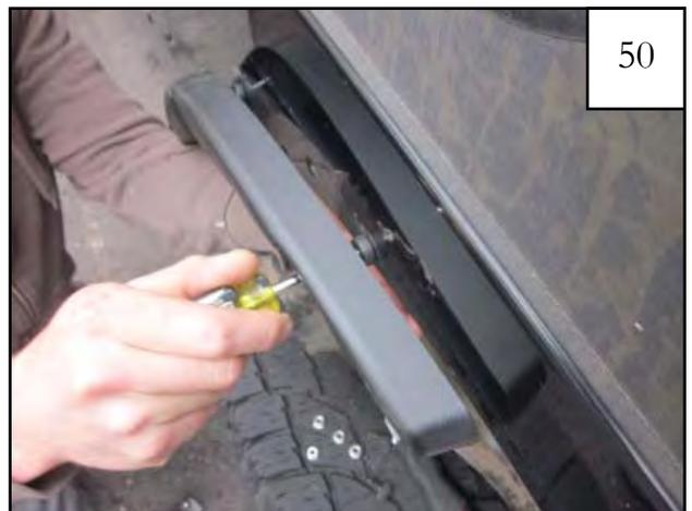
While holding the inner piece in place, use a #2 Phillips bit to tighten the M5-.8 machine screws (SW1-0053) into the flange nuts (NU1-0010).
