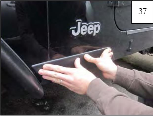
Press rocker piece onto vehicle to promote tape adhesion.
