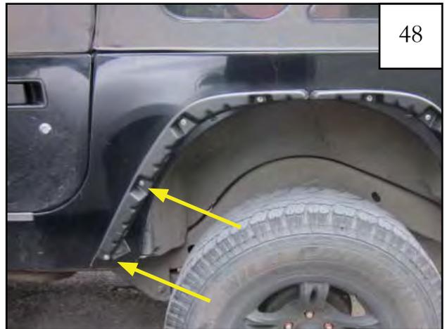
**NOTE: The two bolts on the bottom front of the wheel well do not require nuts.**
