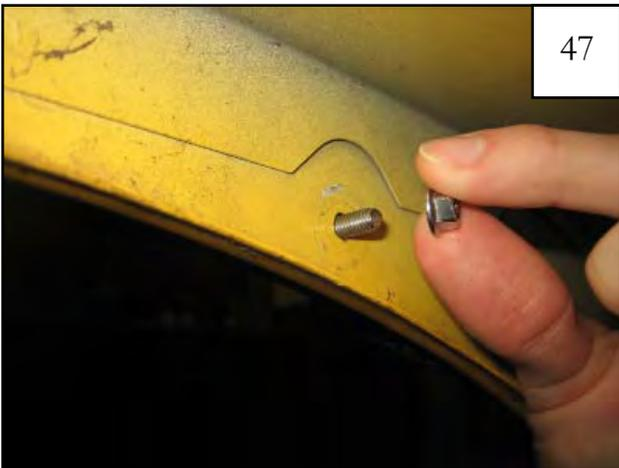
Attach flange nuts (NU1-0010) into the threads on the M5-.8 machine screws (SW1-0053) and hand tighten.
