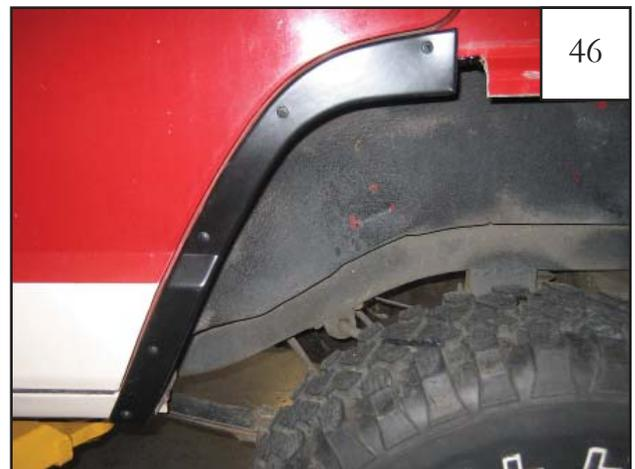
Open door. Install cover piece over "dog leg" using five supplied drill screws (SW1-0066). Place drill screw in indent in part and drill into sheet metal. **NOTE: Some trimming may be required.**
