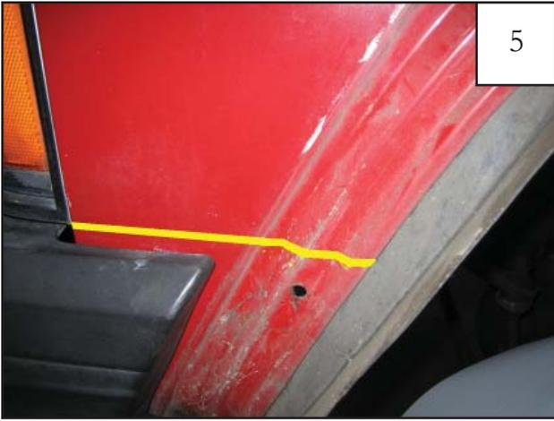
Using a grease pencil, make a horizontal line horizontally from the bottom of the headlight bezel to the inside of the fender well opening.
