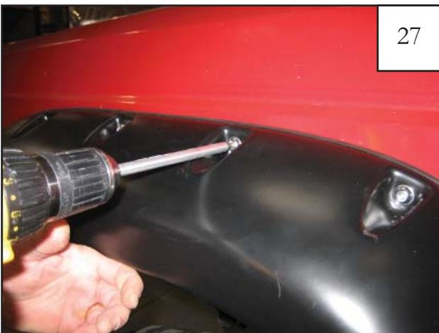
Start each screw with a T45 Torx bit (SW1-0052) in each pocket but do not tighten until all screws have been started. *NOTE: Over-tightening screws may cause them to strip! Use a Torque setting of 24 inch/ounces.*
