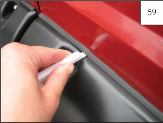
Using flat end of supplied Edge Trim Tool, seat bottom edge of edge trim first by inserting straight flat end between bottom edge of edge trim and part at one open end and slide over entire top edge to the other end.
