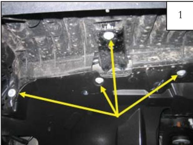
Using a socket wrench with a 10mm socket, remove four factory bolts from inside of splash shield. Set bolts aside for reinstallation.
