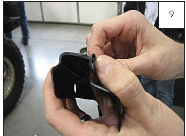
Make sure gimp and inner flare are clean. Peel 2" of liner from gimp (pin shape). Carefully position gimp as uniformly as possible along radius as shown, peeling liner as you go. Gimp can be repositioned as needed.
