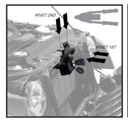
LINE UP THE MOUNTING HOLES IN JK HOOD LOCK WITH EXISTING HOLES ON THE VEHICLE FRAME - USING THE RIVET GUN INSTALL THE 4 RIVETS IN PLACE - START WITH THE 2 FRONT HOLES AS SHOWN - REATTACH HOSE CLAMP
