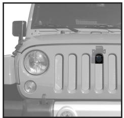
CLOSE AND LATCH HOOD SHUT, TURN KEY TO THE RIGHT TO LOCK THE HOOD AND REMOVE YOUR KEY
