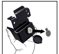
READ AND REMOVE WARNING STICKER - REMOVE KEY FROM KEY CHAIN - KEEP HAND/FINGERS AWAY FROM PIVOTING LOCK ARM WHILE CODING
