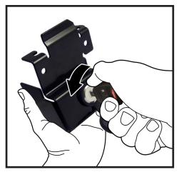
TURN KEY LEFT APROX 1/4 TURN TILL IT STOPS, THE LOCK IS NOW IN THE UNLOCKED POSITION - KEEP LOCK IN THIS STATE DURING INSTALLATION - THE KEY CANNOT BE REMOVED WHILE IN THE UNLOCKED POSITION
