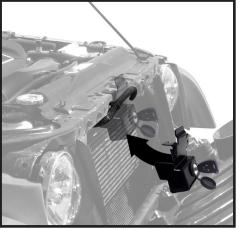
IN THE CENTER OF THE GRILL REMOVE ONE HOSE CLAMP SNAP TO ALLOW THE HOOD LOCK TO BE POSITIONED BEHIND IT
