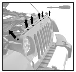
OPEN HOOD; USING A FLAT HEAD SCREWDRIVER REMOVE THE 6 PLASTIC SNAP SCREWS FROM THE TOP OF THE GRILL
