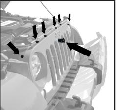
POSITION THE GRILL BACK INTO PLACE USING 6 NEW SNAP SCREWS PROVIDED
