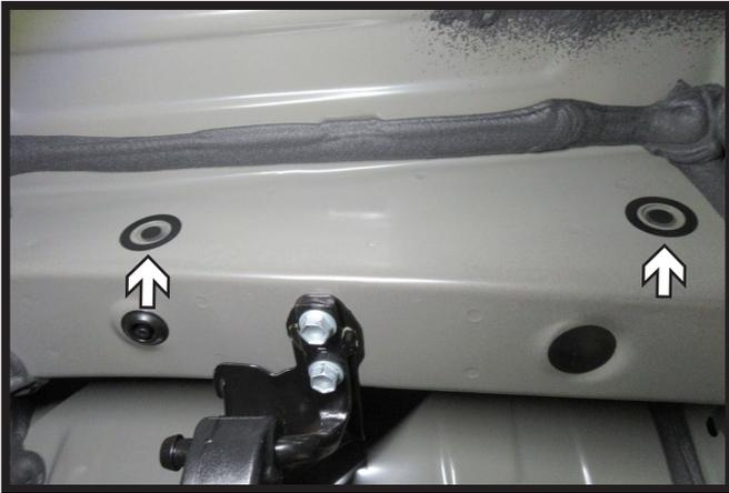
1. Remove the stickers covering the holes in the side for the frame. Do this on both sides of the vehicle.
