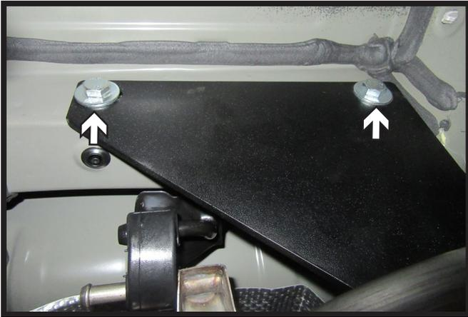
4. Raise hitch into place and install the two (2) M12 bolts with conical washer. Do this on both sides of the vehicle.
