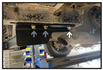
3. Raise hitch into place. Install whiz nut (white) onto 1/2" carriage bolt, leave loose. Then install the two (2) 12M-1.75 bolts (gray) into the existing holes, leave loose. Do this on both sides of the vehicle. **Note**: If needed, lower the exhaust on each side to allow more room to install whiz nuts.
