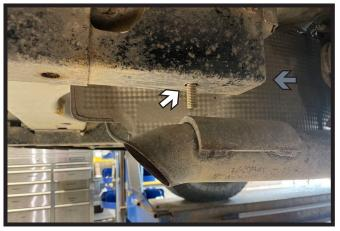
Place spacer plate onto 1/2" carriage bolt. Slide bolt and plate through forward access hole (gray) in the frame. Place bolt (white) in forward hole so that plate is flush with the frame and bolt hangs vertically. Do this on both sides of the vehicle.
