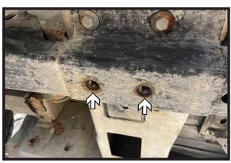
Clean area around existing holes using a wire brush. Then run a 12MM x 1.75 tap through the two (2) holes. Do this on both sides of the vehicle.
