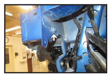
19. Using a 16MM socket, remove the one (1) bolt from behind the bumper on the driver side of the vehicle.
