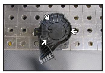
15. Using a T20 Torx, remove the three (3) bolts from the bottom of the pedestrian alert speaker. Remove the mounting bracket from the speaker.
