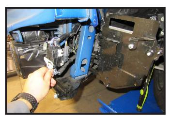
11. Unclip the electrical and wire loom from the front of the black box and the front of the frame on the driver side of the vehicle.
