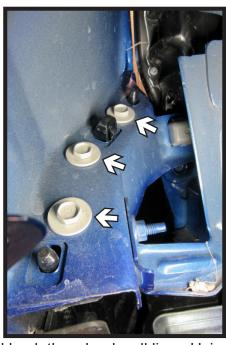
5. Pull back the wheel well liner. Using a 10MM socket, remove the three (3) bolts from the fascia joint. Do this on both sides of the vehicle.
