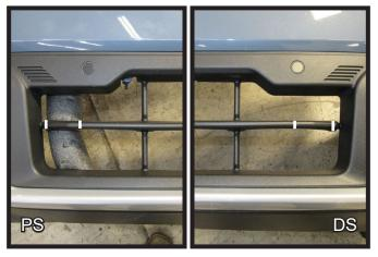
28. Using a reciprocating saw, remove the horizontal slats on each side of the vehicle between the white marks as shown to allow room for the removable tabs.
