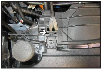
2. Using a flat head screw driver or similar tool, pull up on the plastic piece and outward on the fascia to release clip. Do this on both sides of the vehicle.
