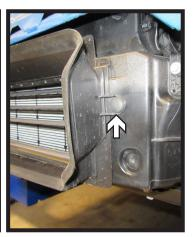
8. Remove the two (2) push pins (white), one (1) on each side of the shroud around the lower shutters. Then using a flat screw driver, release the eight (8) clips around the edge of the shroud (gray). Remove shroud and set aside to be reinstalled later.
