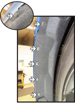
3. Remove the six (6) push pins from the wheel well edge. Do this on both sides of the vehicle.
