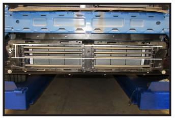
14. Using a reciprocating saw, cut the shutters starting at the top and down 3" to allow for baseplate clearance.
