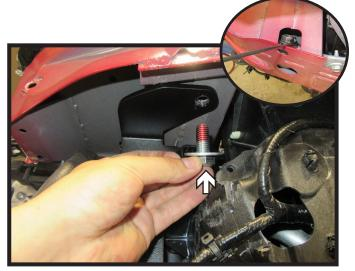
20. Install one (1) 1/2" bolt (white) with flat washer and wire nut (inset).
