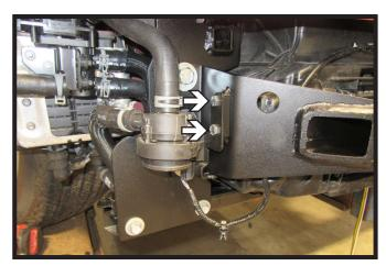
24. Using two (2) 1/4" x 1-1/4" bolts with nuts to attach bracket to the baseplate on the passenger side of the baseplate.
