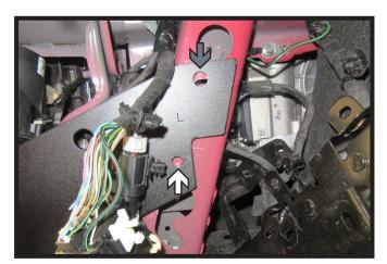
26. Using a 3/8" drill bit, drill out bottom hole in frame (white) on the driver side of the vehicle using the baseplate as a template. Then using a 1/2" drill bit, ream out the top hole in the frame (gray) using the baseplate as a template.
