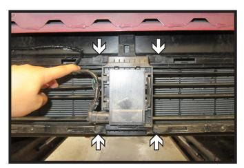
13. Using an 8MM socket, remove the four (4) bolts attaching the Adaptive Cruise Control (ACC) to the vehicle. Let hang out of the way for baseplate installation but DO NOT unplug sensor.
