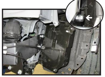
35. Reinstall the black box onto the driver side of the vehicle. Reattach the wire loom to the bottom bolt on the backside. If the box touches the baseplate bolt head, bend back plate slightly to create clearance (inset).
