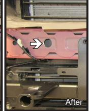
29. Using a 1-1/4" hole saw, drill out the hole as shown to create access hole. Do this on both sides of the vehicle.
