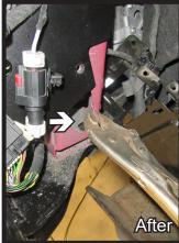
27. Using a pair of large vise grips bend back the frame piece as shown to create an access hole for the nut plate.
