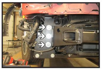
22. On the passenger side of the vehicle, start the three (3) 1/2" x 1-1/2" bolts with washers and nylon lock nuts. Leave loose.
