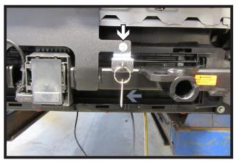
32. **Optional Breakaway**: Put a 90° bend in the breakaway bracket, 1-1/2" from the back and attach to the back of the electrical mounting bracket with provided 1/4" bolt, washers, and nut as shown. Remove white tag (gray) from breakaway switch so it does not interfere with any of the vehicle sensors.
