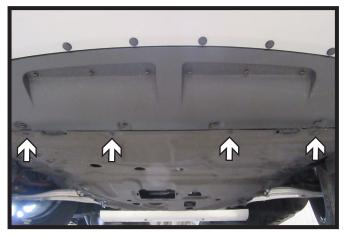
6. Using a 7MM socket, remove the four (4) bolts from the underside of the fascia.
