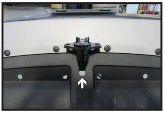
33. Center electrical bracket on bottom of the fascia. Using a 1/4" drill bit, drill two (2) holes using the bracket as a template. Install provided two (2) 1/4" bolts with hardware (left). Hold electrical plug in place and mark fascia below end of plug. Using a 5/8" drill bit, drill one (1) hole to feed tail light electrical wires through (right).
