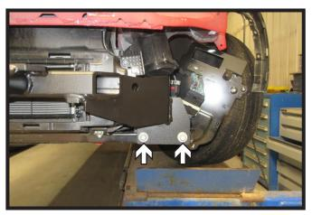
21. Slide baseplate onto vehicle. Start the two (2) existing bolts with washer into the bottom holes on the driver side of the vehicle. Leave loose.
