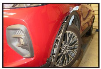
Pull back the wheel well trim past the fascia joint and hold in place with a soft cloth. Do this on both sides of the vehicle.
