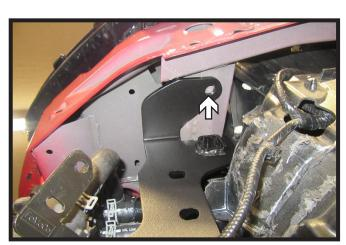
19. Using a 1/2" drill bit, drill hole in frame using the baseplate as a template.
