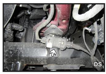
4. Unplug the one (1) electrical connection on each side of the vehicle.
