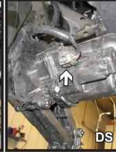
10. Using a 13MM socket, remove the two (2) nuts from the automatic valence. Do this on both sides of the vehicle. Unplug the electrical connection on the driver side and remove valence and set aside to be reinstalled later.
