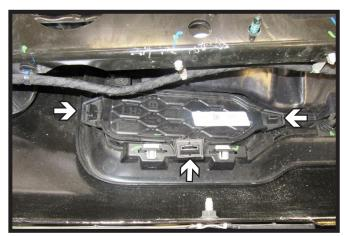
Vehicles without Tow Hooks: Unclip the three (3) clips from the tow hook cover and push towards the back of the bumper to remove. Do this on both sides of the bumper.
