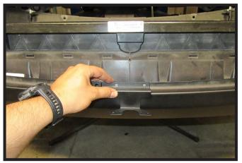
Rebel/RHO Models: Hold electrical bracket on top of the bumper/fascia and mark holes. Using a 7/32" drill bit, drill two (2) holes.
