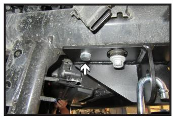
Install the 1/2" x 1-1/2" bolt with lock washer and whiz nut into the bottom back hole. Fully tighten all bolts at this time starting with the side bolt, then back bottom bolt, and finally the front bottom bolt. Do this on both sides of the vehicle.
