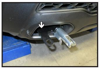
16. Non-Rebel/RHO Models (Optional): Attach breakaway switch to the hole in the convenience link using the provided hardware.
