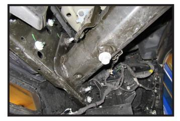
Trucks with Tow Hooks: Remove rubber grommet (white) and metal piece (gray) from back tow hook bolt. Reinstall the tow hook bolt and hardware. Do this on both sides of the vehicle.
