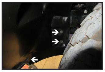
1. Using an 8MM socket, remove the five (5) bolts from the wheel well. Do this on both sides of the vehicle.
