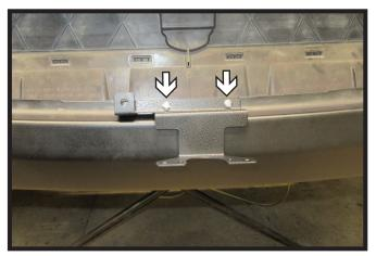
12. **Rebel/RHO Models**: Install electrical bracket to the top of the bumper/fascia using the provided hardware.
