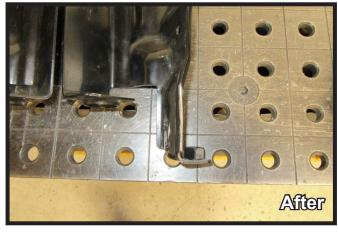
3. **RHO Models**: Using a reciprocating saw, cut along the weld at the bottom of the belly pan bracket. Remove piece from bracket. Do this on both brackets.
