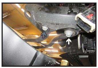
1. Trucks with Tow Hooks: Using a 21MM socket remove the front bolt (gray), and then using an 18MM socket remove the back bolt (white) attaching the tow hook to the frame. Remove tow hook. Do this on both sides of the vehicle. The tow hooks will not be reinstalled.
