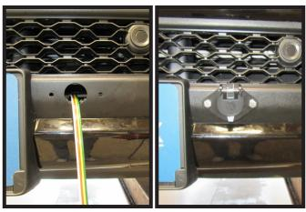
15. **Non-Rebel/RHO Models**: Using a 1-1/2" hole saw drill a hole in the bumper on the driver side for the electrical plug as shown. Hold plug in place, using a 1/4" drill bit, drill the two (2) holes in the bumper for the bolts using the plug as a template. Install plug using provided hardware.
