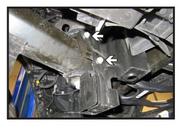
RHO Models: Using a 13MM socket, remove the two (2) bolts from the belly pan bracket. Remove bracket and set aside to be reinstalled later. Do this on both sides of the vehicle.
