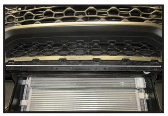
5. Using a reciprocating saw, cut a straight line (white line) across the plastic piece to remove the indicated area.
