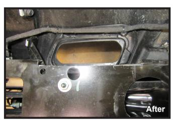
12. In necessary, use a reciprocating saw to trim the indicated area from the metal piece on the back of the bumper as shown. Do this on both sides of the vehicle.
