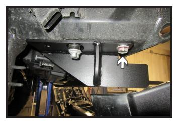
6. Raise baseplate into place and start the 14MM bolt with flat washer and nylon lock nut, hand tighten. Do this on both sides of the vehicle.
