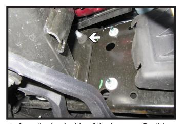
5. Using an 18MM socket, Remove the three (3) nuts from the back side of the bumper. Do this on both sides of the vehicle.
