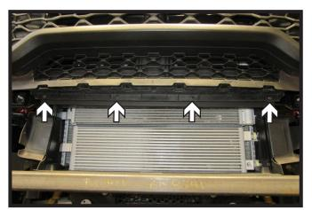
Remove the four (4) push pins from rubber piece below grille and remove. It will not be reinstalled.
