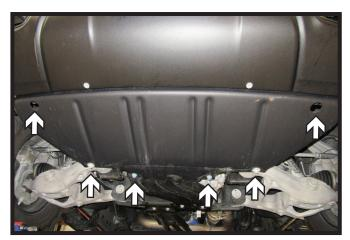
2. **RHO Models**: Using a 16MM socket, remove the six (6) bolts from the belly pan. There are four (4) along the back and two (2) in the front. Remove belly pan and set aside to be reinstalled later.
