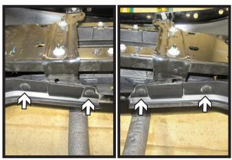
5. Remove the four (4) push pins, two (2) on each side, from the rubber piece on the top of the bumper.
