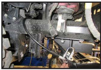
10. Attach the permanent baseplate safety cables to the provided convenience link on the baseplate. The photo above shows the recommended installation of the cables to frame of vehicle. Additional options may interfere with suggested mounting; in this case, secure the cables to a solid piece of the frame as described in the General Information sheet. Be sure the safety cables do not rub against any hoses or moving parts. Do this on **BOTH** sides of the vehicle.
