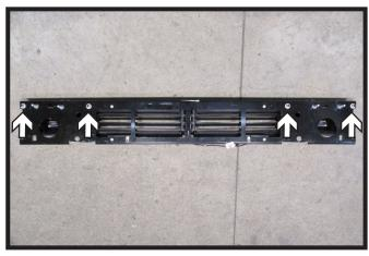
17. Using a 10MM socket, remove the four (4) bolts attaching the shutters to the bumper frame. Remove shutters and set aside to be reinstalled later.
