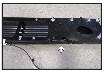
15. Using a reciprocating saw remove the marked area as shown. Be careful not to cut the wire loom attached to the bumper. Do this on both sides of the bumper.
