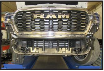
25. Reattach the shutter housing to the shutters and reinstall the lower shutters onto the bumper frame.
