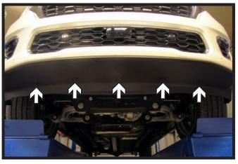
5. Using a 10MM socket, remove the five (5) bolts from the bottom of the fascia.
