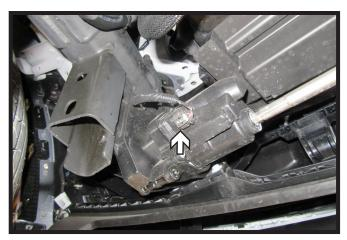
6. Unplug the electrical from the automatic valence on the driver side of the vehicle.
