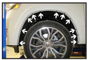
Using an 8MM socket, remove the eleven (11) bolts from the wheel well trim. Do this on both sides of the vehicle.
