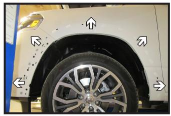
2. Pull trim outward to release from clips and remove. Set trim aside to be reinstalled later. Remove clips and attach them to trim for easier reinstallation. Do this on both sides of the vehicle.
