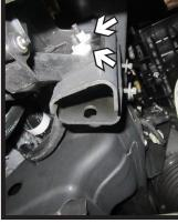
Using a 13MM socket, remover the four (4) nuts, two (2) on each side. Remove valence and set aside to be reinstalled later.
