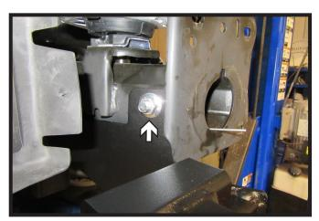
20. Start the one (1) 1/2" carriage bolt with plate and whiz lock nut in side hole of the baseplate. Tighten bottom bolt then side bolt. Do this on both sides of the vehicle.
