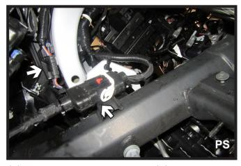
10. Unplug the three (3) electrical connections, one (1) on the driver side and two (2) on the passenger side, from behind the bumper.
