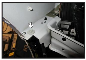
4. Using a 10MM socket, remove the one (1) bolt from the fascia joint. Do this on both sides of the vehicle.
