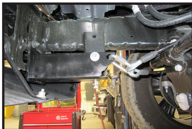
6. Attach the permanent baseplate safety cables to the provided convenience link on the baseplate. The photo shows the recommended installation of the cables to frame of vehicle. Additional options may interfere with suggested mounting; in this case, secure the cables to a solid piece of the frame as described in the General Information sheet. Be sure the safety cables do not rub against any hoses or moving parts. Do this on **BOTH** sides of the vehicle.
