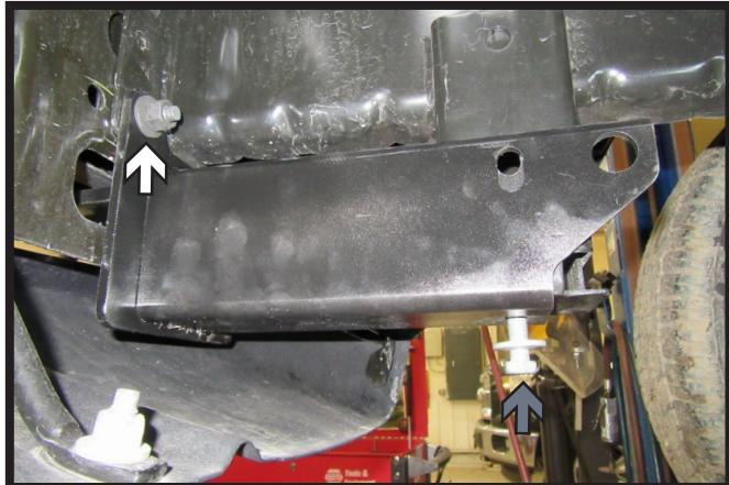
4. Install the baseplate onto the frame. Reinstall the existing nuts (white) and bolt (gray), fully tighten all hardware. Do this on both sides of the vehicle.
